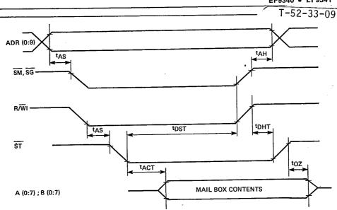
FIGURE 7 — INTERNAL BUS — FROM MAIL BOX TO PAGE MEMORY OR CHARACTER GENERATOR OR VIN TRANSFER CYCLES
