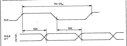
FIGURE 3 - R, G, B and I TIMING (VIN)
