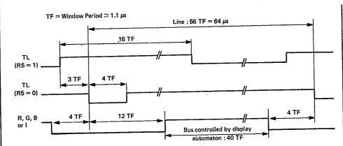
$\dot{2}62$  line periods (if R6 = 0) or 312 line periods (if R6 = 1) make a frame period. The TT output is at frame period (60 Hz/50 Hz) and is low during 2 lines. SYT input resets the line count inside the frame : this input is triggered, then sampled when the 12th window of each line occurs. When the sample transits from 1 to 0, the line count will be reset on the next TL.
